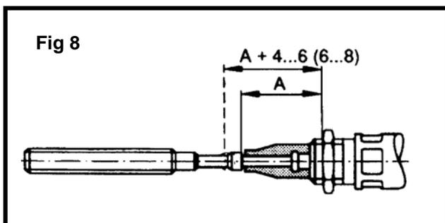
The free play should be as uniform as possible for 2 or 4 wheel brakes respectively.
