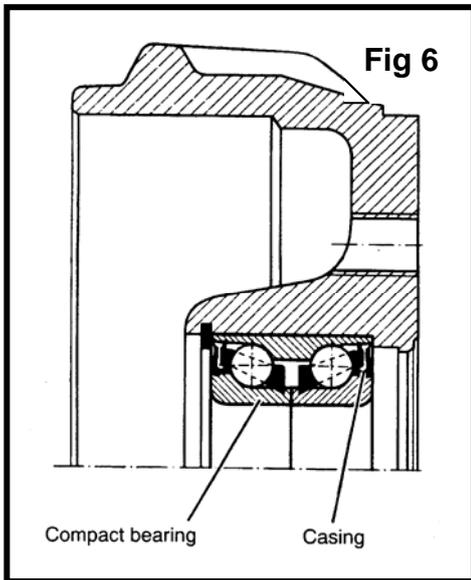
The wheel bearing is a double-row inclined ball bearing. It has the following advantages over normal bearings.
