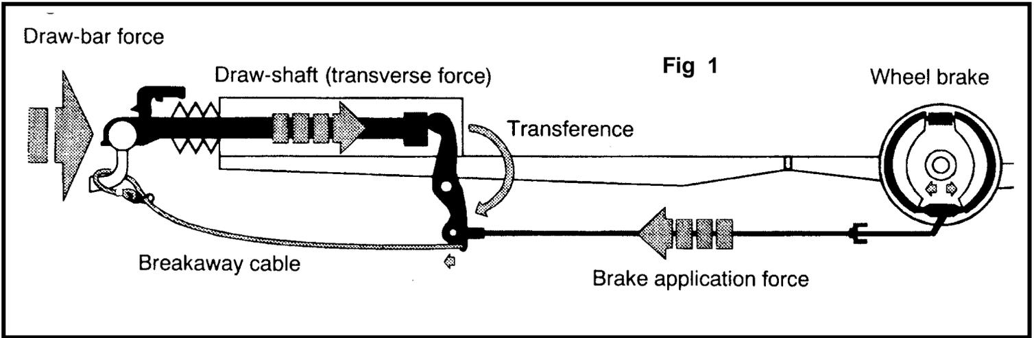
The overrun device can be described as the control device of the overrun brake system. A draw-bar force is produced at the coupling point by reducing the speed of the towing vehicle. After the threshold level has been passed, the draw shaft is pushed in, thus actuating the overrun lever, the wheel brakes (1 & 2) are then applied via the expanding clutch (3) (Fig 2)
